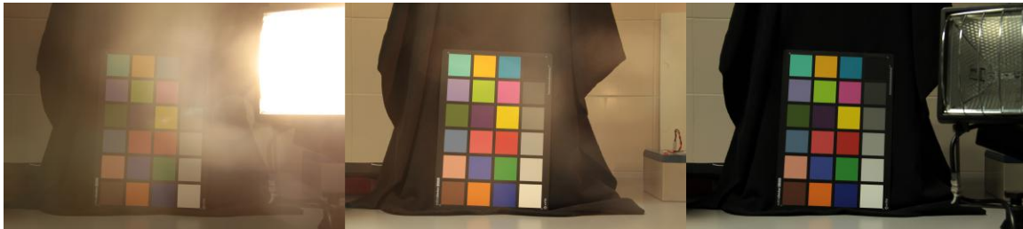
Figure 5-4: Scenes captured with different veiling glare conditions to test the influence of this phenomenon in the calculation of CRF . From left to right, scenes 1 to 3.
