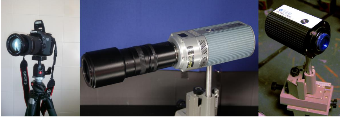
Figure 4-3: Left: Canon EOS 7D commercial RGB camera. Center: Retiga SRV 1300 monochrome scientific camera. Right: Retiga 1300 C , RGB scientific camera.
