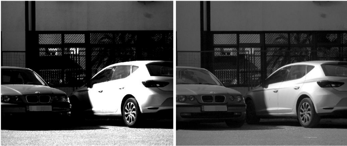
Figure 5-33: Grayscale images of scene 1 (see figure 5-31) captured at 555 nm with a bandwidth of 50 nm and polarization angle 0°. Left: LDR image. Right: tonemapped HDR image.
