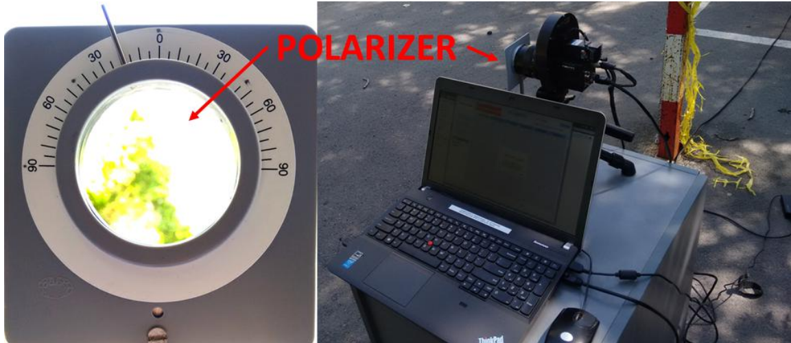
Figure 5-23: Spectrocam set up used for capturing outdoor scenes with a linear polarizer attached to a goniometer in front of the camera.
