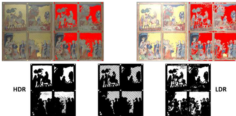
Fig. 8. RGB renderization of the spectral reflectance cubes, together with red highlight of the golden material found, and the segmentation compared with the ground truth. Left: Cube_{HDR} . Right: Cube_{LDR} .
