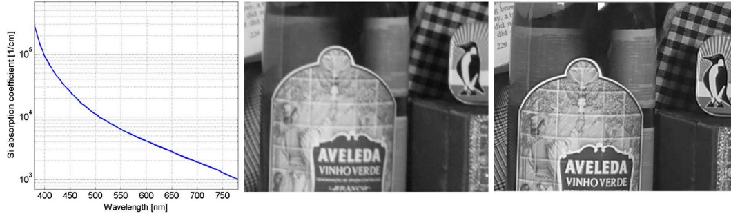
Figure 3: Left: Wavelength dependency of the absorption coefficient of silicon. Center: luminance image retrieved from an image taken with a Bayer-filtered sensor. Right: luminance image retrieved from an image taken with a Sony Foveon X3 sensor
