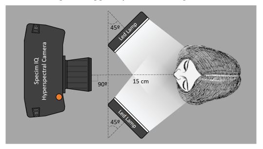
**Figure 1.** Schematic representation of the measurement set-up used to measure the hyperspectral reflectance images of the four maxillary incisors.
